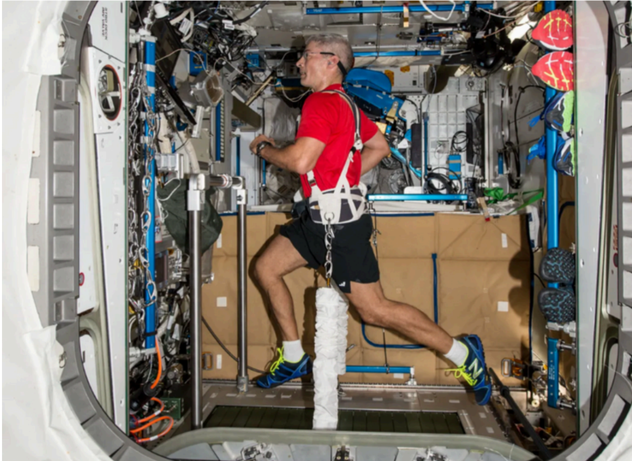
Image Credit: NASA – Astronaut Mark T. Vande exercising on the Combined Operational Load Bearing External Resistance Treadmill in the International Space Station.
